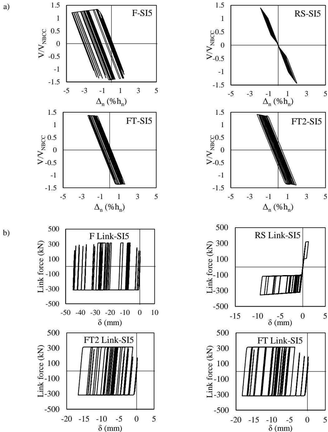
Figure 7. a). Storey shear vs storey drift hysteretic responses of the systems b). Load vs. deformation response of the friction dampers (links) of the systems
