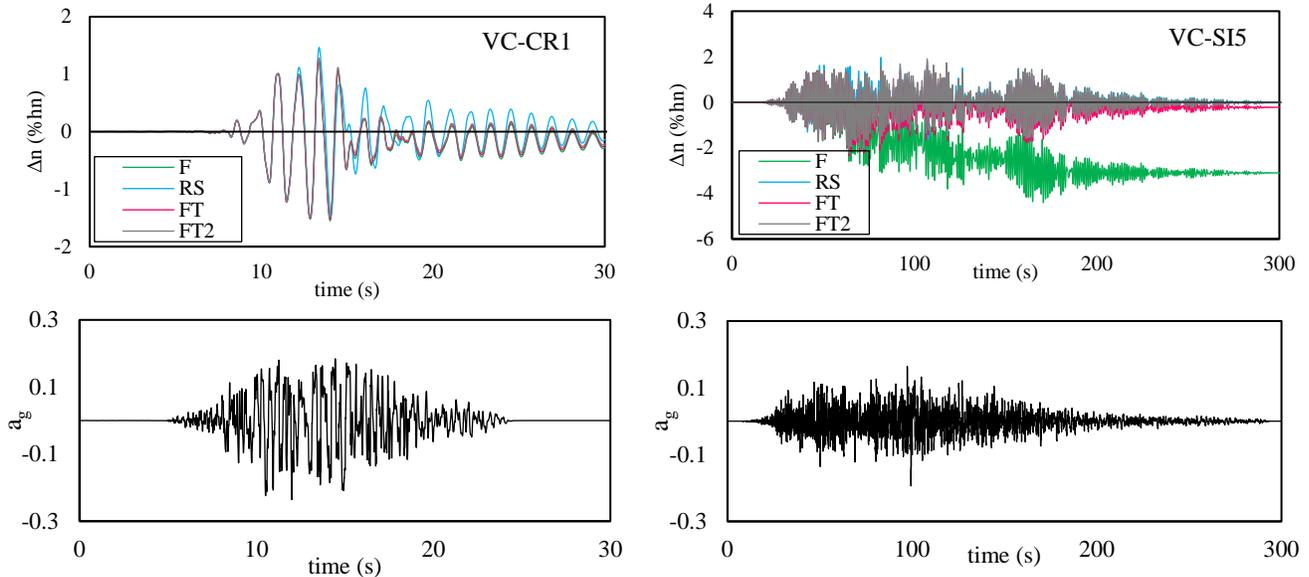
Figure 6. Time history response of the roof displacements under crustal and subduction interface ground motion records.
