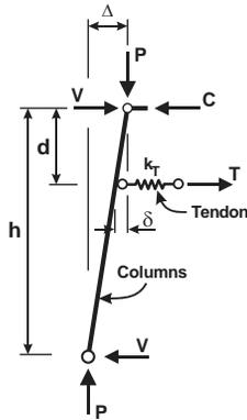
Figure 3. Equilibrium of the FT-TMF system upon activation of the dampers.
