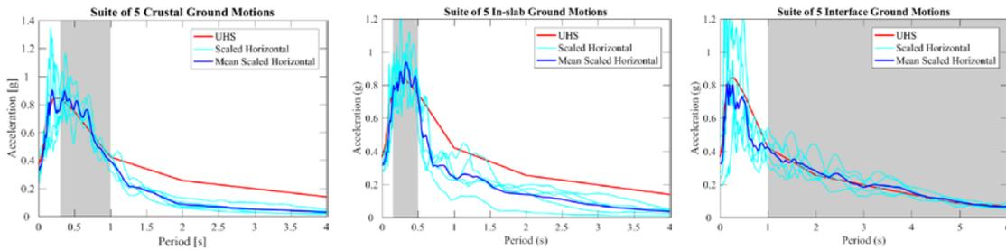
Figure 5. 5% damped spectra of the ground motion records of each suite.
