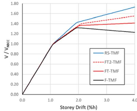
Figure 4. Load-deformation responses of the TMF systems studied
