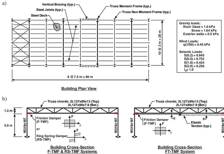
Figure 2. Building studied: a) Building plan view and design loads; b) Building cross-sections illustrating the F-TMF, RS-TMF and FT-TMF systems.
