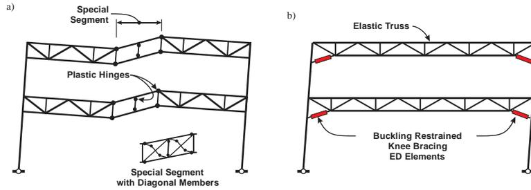
Figure 1. Truss moment frame systems: a) Conventional configuration with a yielding segment; b) Newly proposed configuration with buckling restrained knee-bracing energy dissipation elements.
